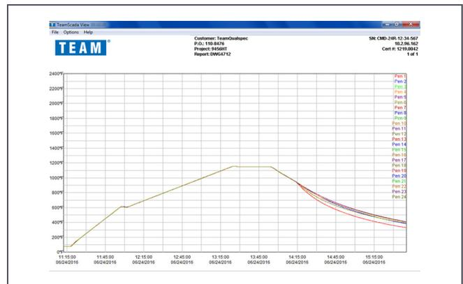
**Trend Chart:** Printed charts can be configured with multiple options including orientation, time interval and which pens to display. The hard-coded job information in the header ensures data integrity for traceability of performed jobs.
