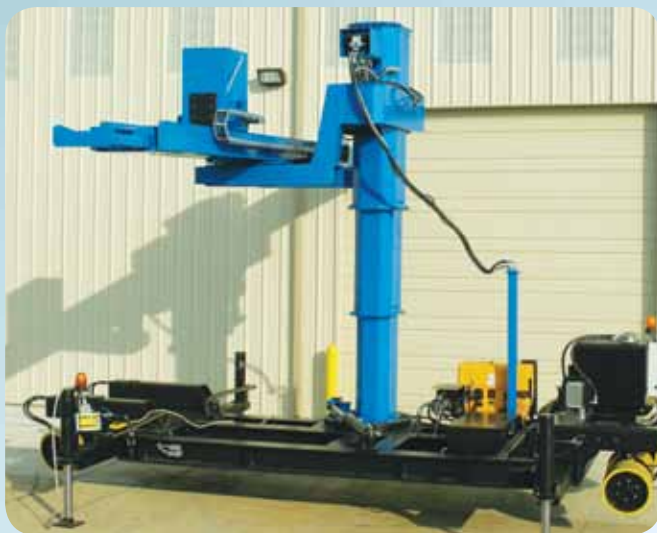
Crawler extractor for bundle exchangers up to 30-feet long and 60,000 pounds.
